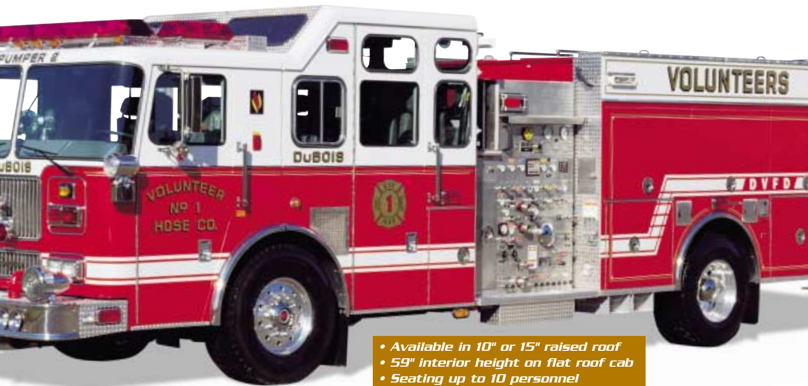
Removable wheel well liners on both cab and body and optional removable outer wheel well panels
