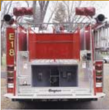
Ultra-low hose bed floors starting at 42 inches from the ground
