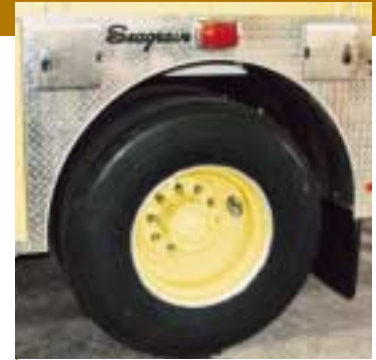
Removable wheel well liners on both cab and body and optional removable outer wheel well panels
