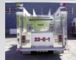
Enclosed Ladder and Suction Storage
